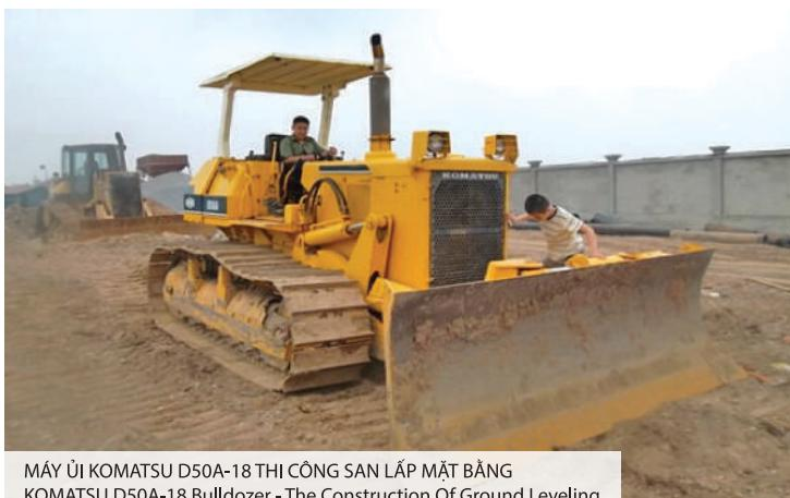
MÁY ỦI KOMATSU D50A-18 THI CÔNG SAN LẤP MẶT BẰNG
