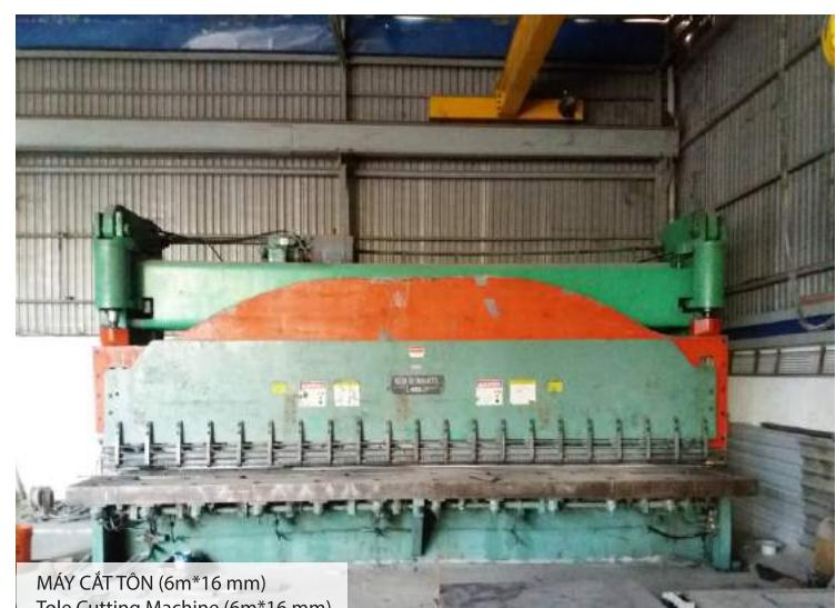
MÁY CẮT TÔN (6m\*16 mm)
